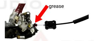
STEP 4 Align EASYPOP cable to geometry on latch that is identifiable.
